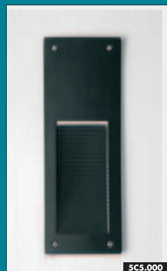
Recessed luminaries suitable for installation in walls or in step risers. Made in shockproof POLYCARBONATE material, UV rays stabilized, rust and corrosion free. No maintenance or painting required. Insulation class II, protection rate IP 66. Modular front cover system. Version with LED plate or with compact fluorescent lamp available.
