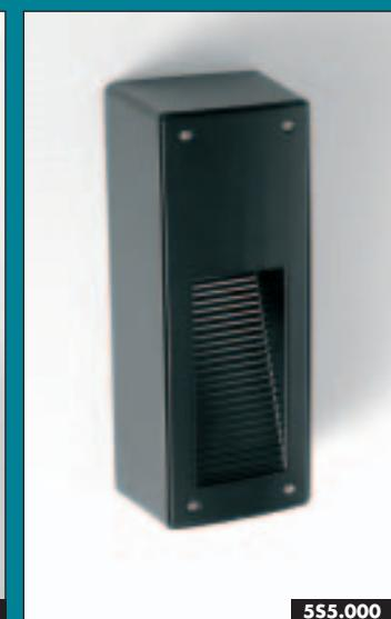
Wall and ceiling surface mount luminaries made in shockproof POLYCARBONATE material, UV rays stabilized, rust and corrosion free. No maintenance or painting required. Insulation class II, protection rate IP 66. Modular front cover system. Version with LED plate or with compact fluorescent lamp available.
