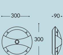
High energy efficiency : the LED version of "Lucia" bulkhead supplies an increased amount of light with reduced consumption compared to traditional light sources.
